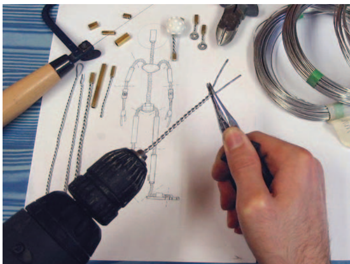
Figure 5.13 Twisting wire in a drill. Courtesy of ScaryCat Studio
