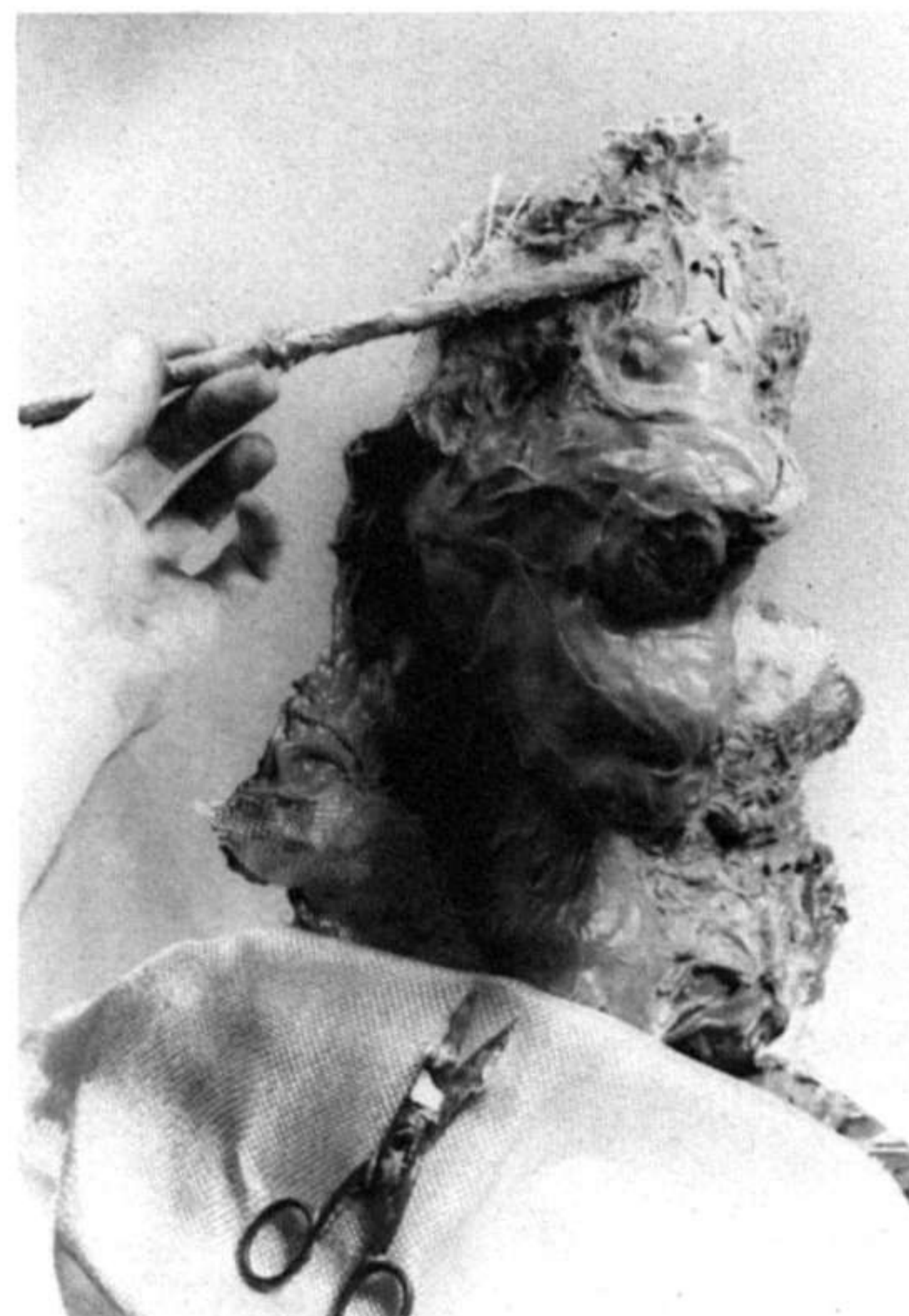
8. The edges of the mold (seam walls) are reinforced strips of fiberglass cloth.
