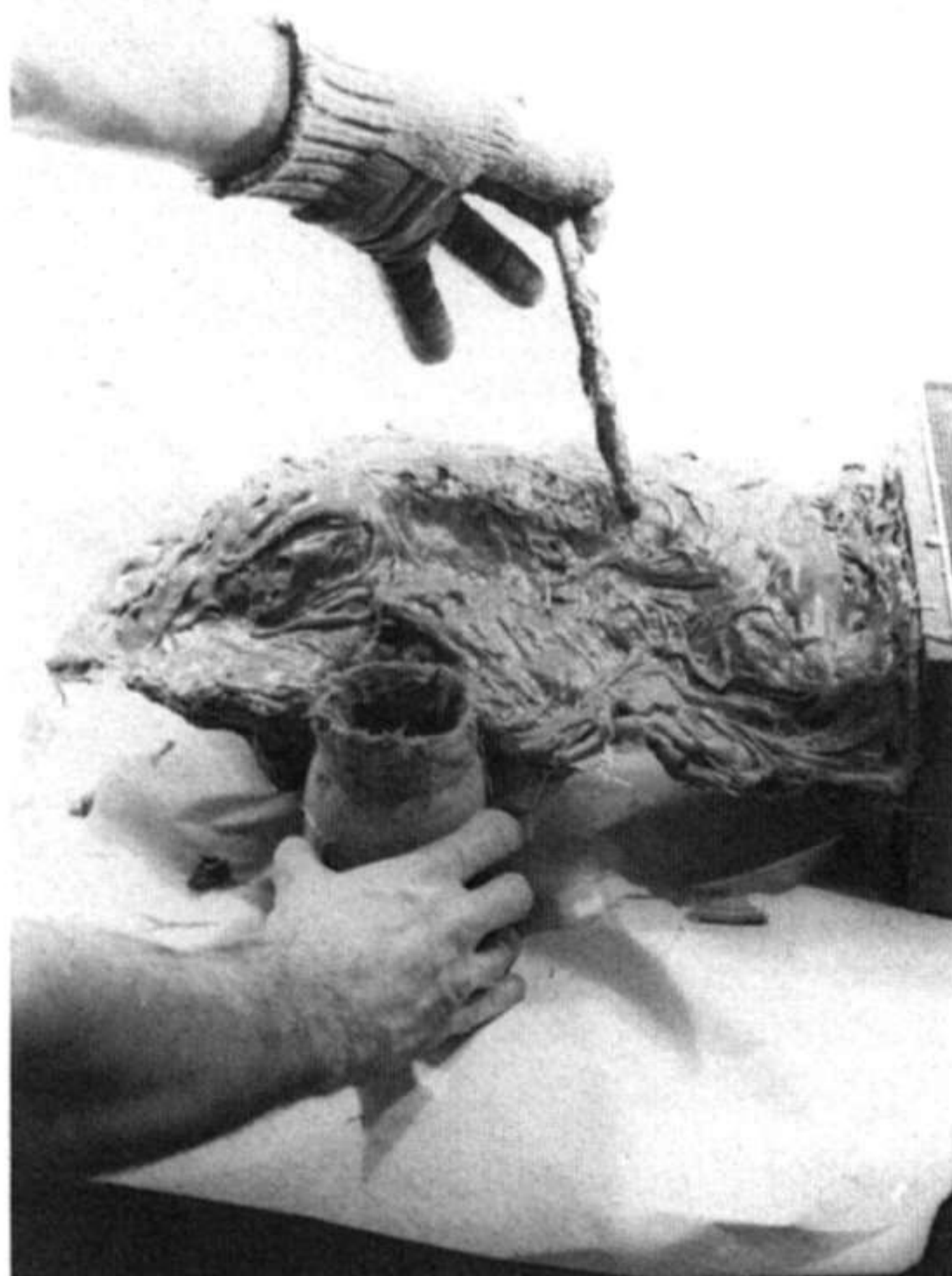
13. Applying the Duraglass (fiberglass and plastic), which is the second coat. The edges are again reinforced with fiberglass cloth.
