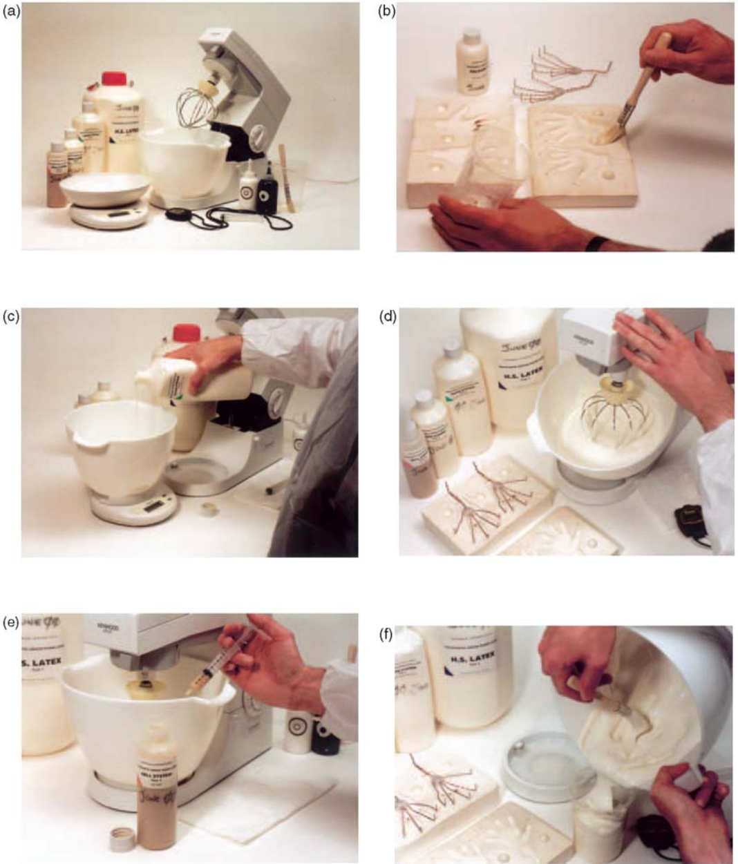
Figure 6.12 Sequence of photos mixing and casting with latex. (a) Materials needed for making foam latex. (b) Brushing on release agent. (c) Measuring latex. (d) Mixing foam. (e) Adding gelling agent. (f) Pouring the mixed foam into the mould. (g) Filling the mould with a brush to release large air bubbles. (h) Closing the mould. (i) Pressing mould halves together. (j) Weighing down the mould. (k) Putting the mould in the oven. (l) Trimming the mould. (m) Removing the new cast. (n) Trimming spare latex. (o) Snipping armature wires. (p) Sponging on paint. (q) Painting on details. Courtesy of John Parsons. Photos © Susannah Shaw
