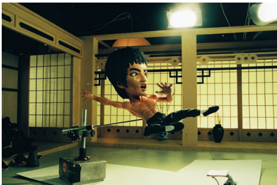
Figure 7.8 Climpex used to make a rig. Set by Artem, model by Mackinnon & Saunders. © Bob Thorne, Artem Ltd/Brisk Tea/JWT
