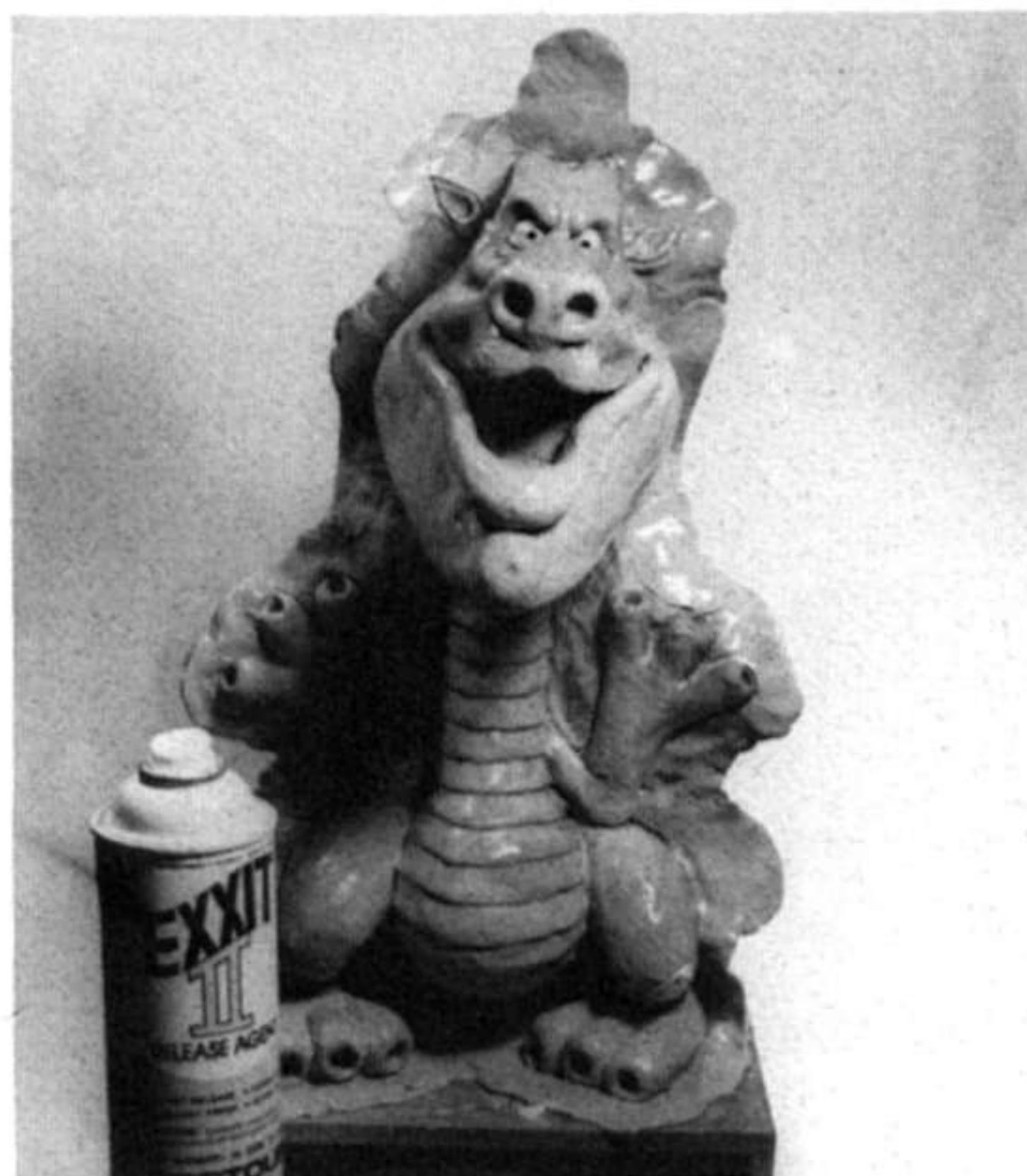
2. The model is sprayed with Exxite II release agent. Apply liberally to prevent the plastic materials sticking to the clay.
