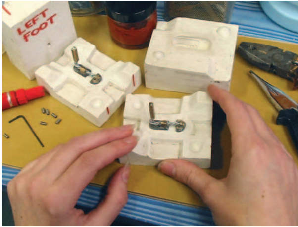
Figure 5.24 Foot armature in mould. Courtesy of ScaryCat Studio
