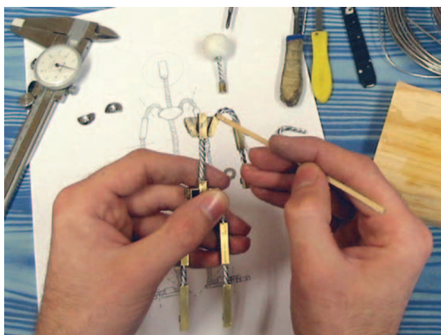
Figure 5.14 Gluing the wire armature. Courtesy of ScaryCat Studio
