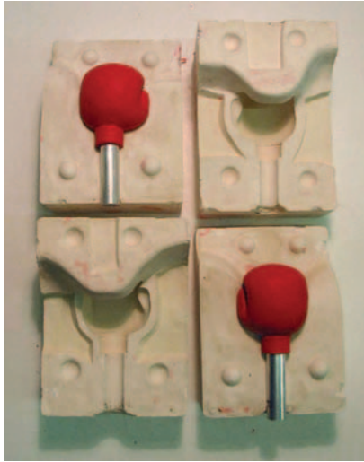
Figure 6.11 (a) Body mould. (b) Glove mould. Courtesy of ScaryCat Studio
